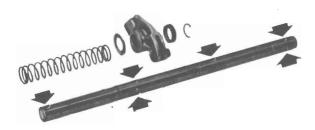
IMPORTANT — Make sure that the shafts are located correctly. Note the difference between exhaust and intake side. Check that oil channels in shaft will align with the head, while at the same time the recess for cyl. head bolts are correctly positioned.
