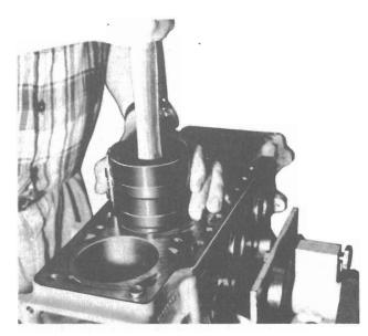
NOTE: The piston crown arrow marking should point towards the front (timing gear end) of the engine
